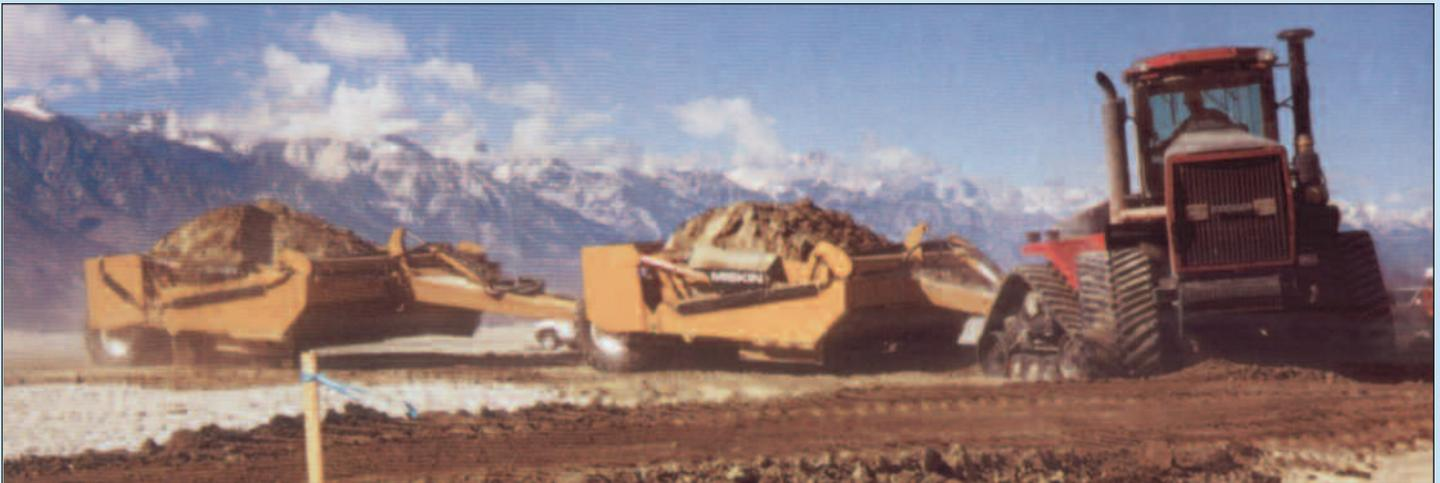
***IN THE '30S, most scrapers were drawn by crawler tractors, but early motor scrapers were just entering the market. As with the loaders, most scrapers of the period were cable-operated from control units mounted on the back of the tractor or prime mover. Ironically, in the 1990s tractor-pulled scrapers had a resurgence, with one to three hydraulic scrapers behind large rubber-tired or rubber-belted tractors (above).***
